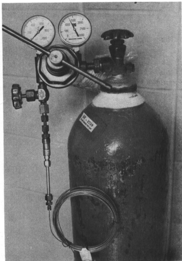
FIGURE 1 Apparatus For Coating PLOT Columns
